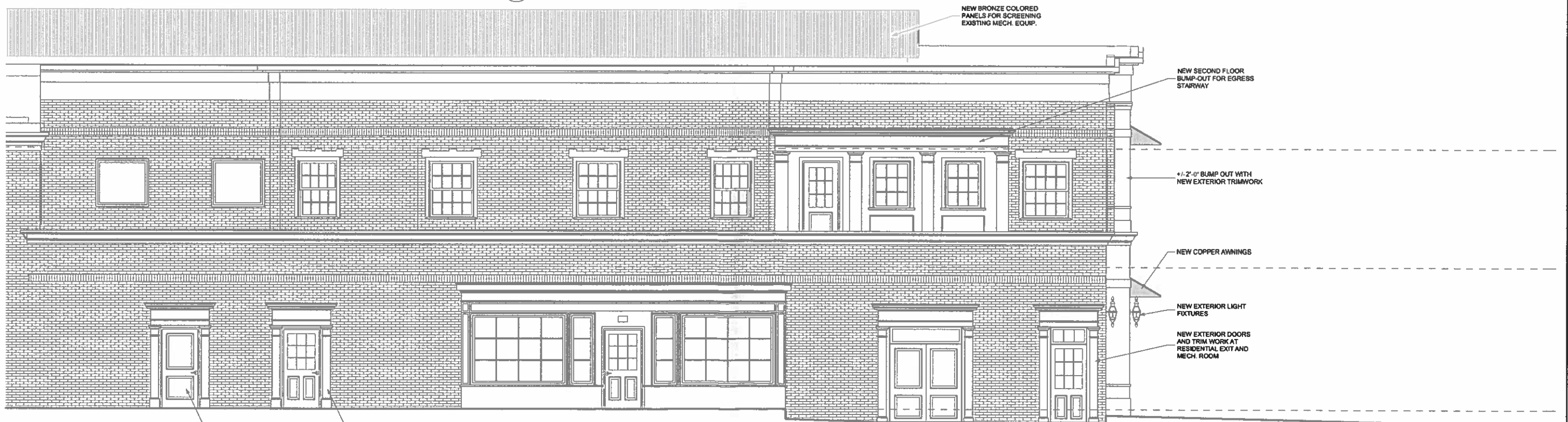
2 EAST ELEVATION - PROPOSED SCALE: 1/4" = 1'-0"
