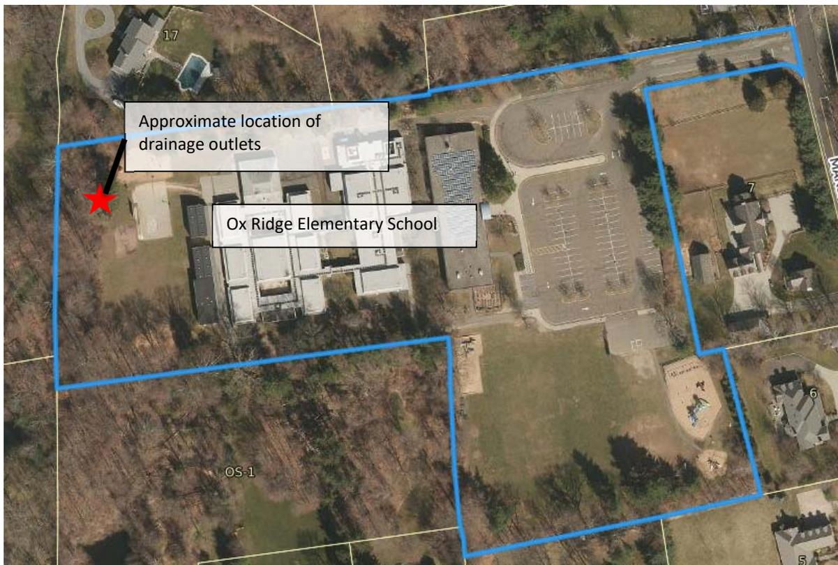
The site slopes from east to west with terraced landforms to accommodate the existing building. The slope varies at about 10% slope at the access drive to Mansfield Avenue, 4.5% slope at the eastern parking lot, 3% at the southeastern field and 2% at the western field. At the western edge of the site, at the edge of the woodland corridor, the grade steeply drops at about 40%.
